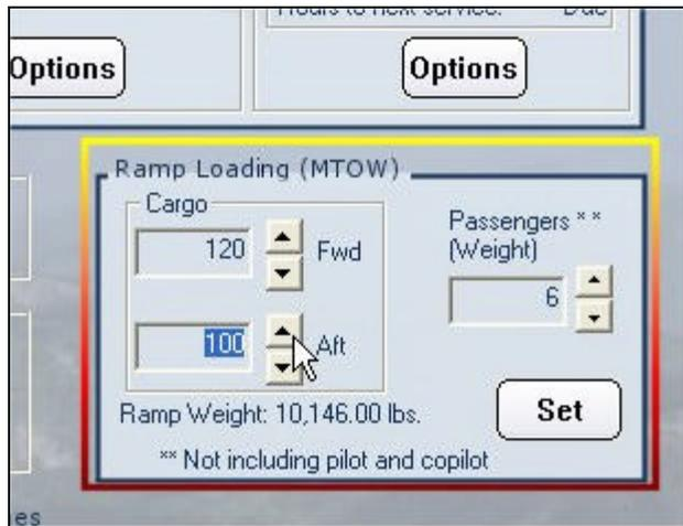
The maximum recommended ramp weight for the Cheyenne is 12,135 lbs., including cargo, passengers and fuel. The Load Manager calculates the ramp weight under the condition of a full fuel load, which is how Flight Simulator typically loads an aircraft. If you are over this recommended weight you will see the following warning issued:
